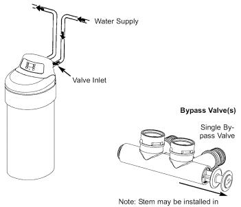
Note: Stem may be installed in either direction. The end with writing should be pulled out for service position.
